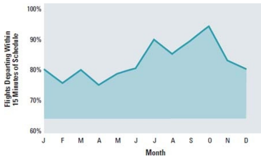
Figure 14.12 Control chart for departure delays showing percentage of flights departing within 15 minutes of schedule
