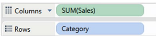
Figure 3-61. Dimension “Category” placed on the rows shelf and the measure “Sales” placed on the columns shelf
